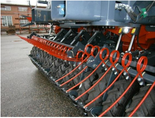
Picture 35: Rear harrow position before folding to driving position
