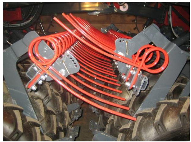
Picture 36: Rear harrow locking dowels in driving position
