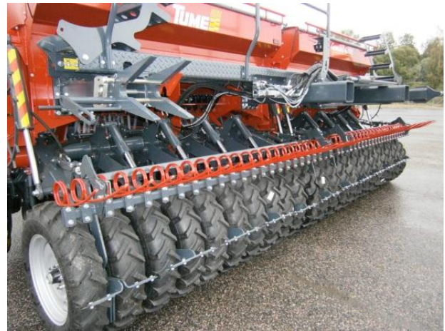
Picture 32: Rear harrow raised in the machine's seeding position
