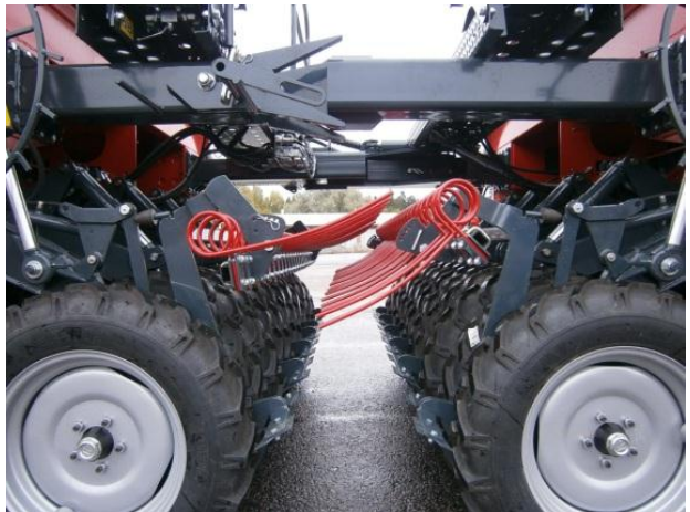
Picture 38: Rear harrow in driving position.
