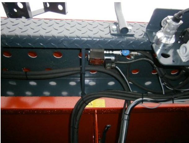
Picture 33: Rear harrow's control valve
