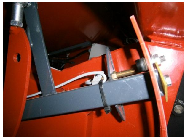
Picture 34: Control of the moment the rear harrow is raised
