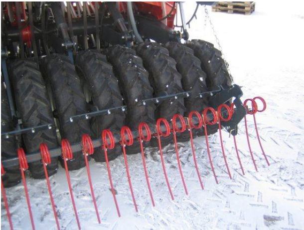
Picture 31: Rear harrow in seeding position
