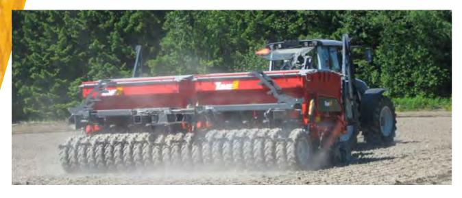
Tume has already over ten years experience of wide working width seed only and combined seed and fertiliser drills. As example of wide drill models of those days was Tume Maximaster of 8 m working width.
