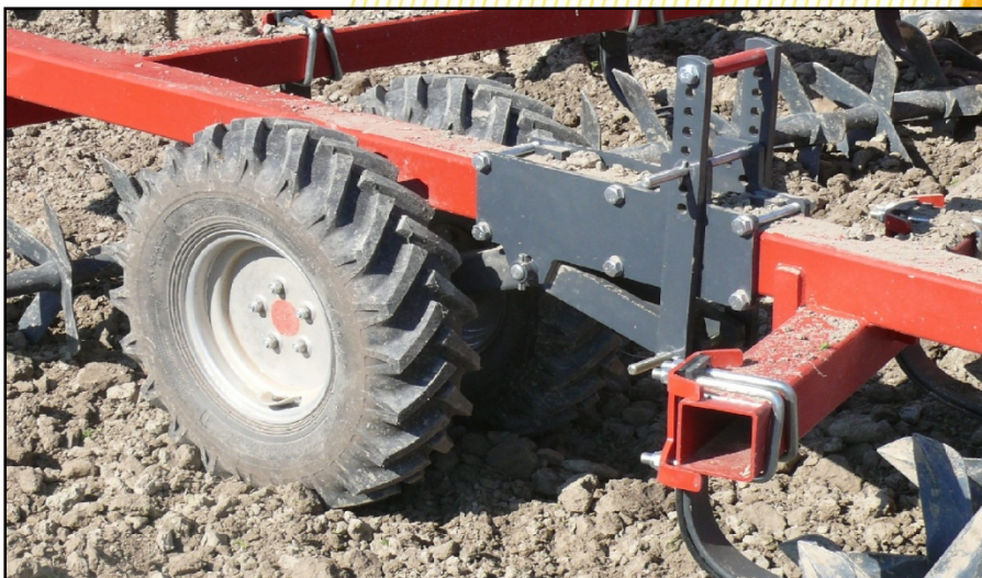
Knife axle bearing construction in models 3800-4600-6400
