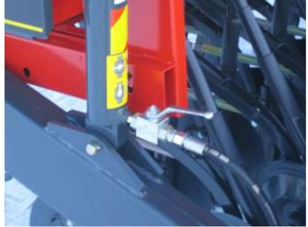
Figure 35. Lift cylinder safety valve open
