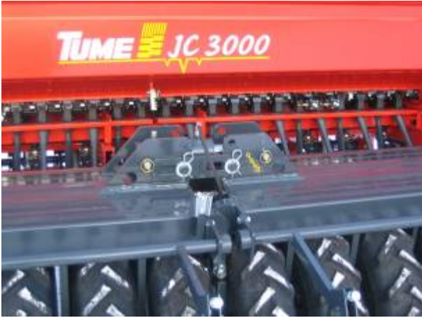
Figure 4. Adjustable joint restriction and locking bar
