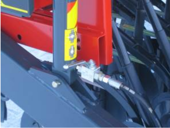
Figure 34. Lift cylinder safety valve closed
