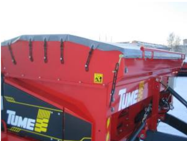
Figure 12. Tarpaulin cover in work position
