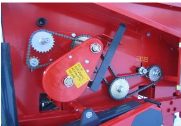
Figure 18. Power transmission cassette I = GRAIN
