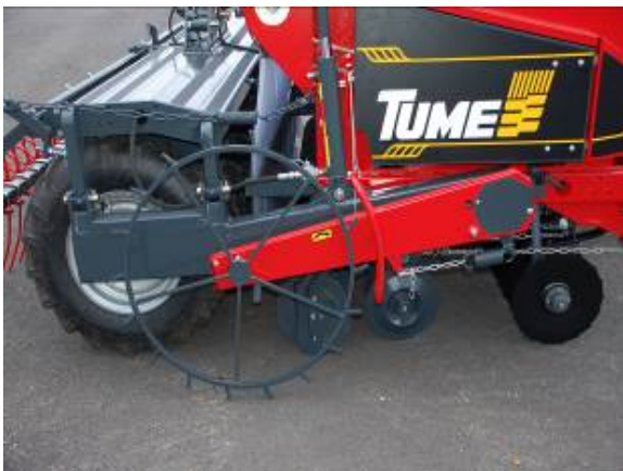
Figure 10. Ground-wheel in work position
