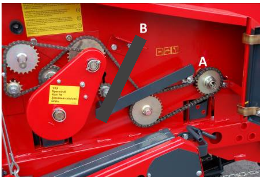
Figure 26. Using the seed side rotation test system Simultaneous rotation test for fertilizer and seed
