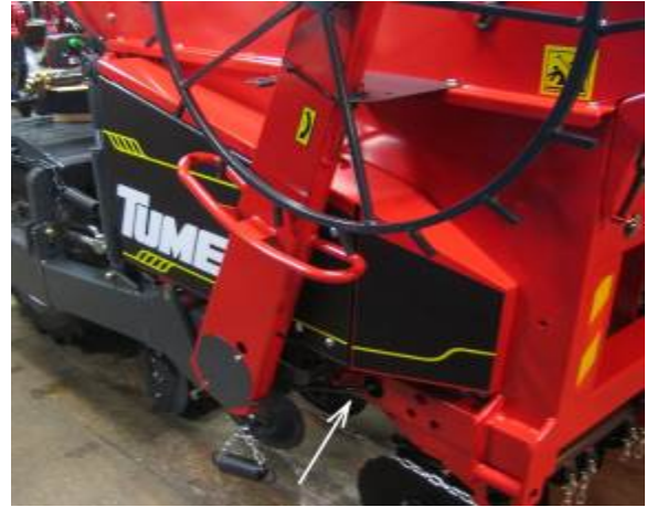
Figure 5. Ground wheel in vehicle transport position
