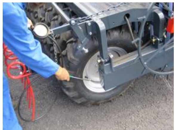
Figure 41. Checking the tire pressure
