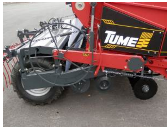
Figure 11. Ground-wheel in transport position
