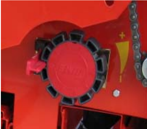
FIG. 9. Feeder adjustment with handwheel
