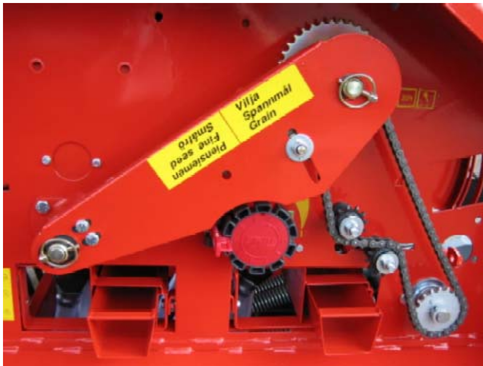
FIG. 11. Transmission cartridge. I = Grain, II = Small seed
