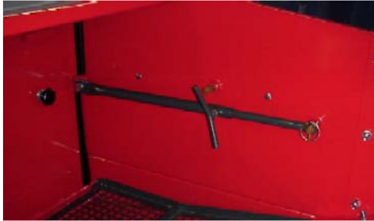
Fig. 8. Container partitioning wall control rod.
