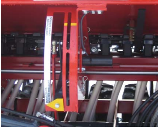
FIG. 4. Control indicator element NOTE: IF THE MACHINE IS LIFTED SO, THAT ELECTRICITY IS NOT CONNECTED, THE YELLOW POINTING ARROW MUST NOT RISE PAST THE LIMIT MARK
