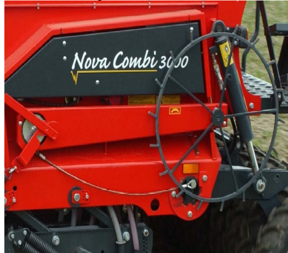
Fig. 7: The ground wheel in transport position
