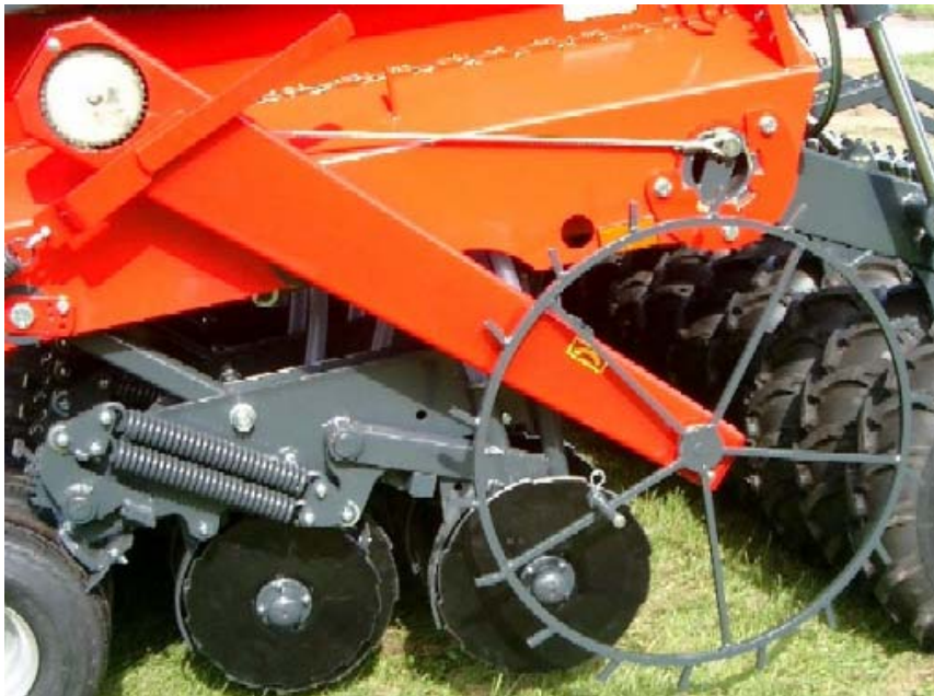
FIG. 14. Ground-wheel in calibration position
