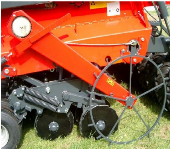
Fig. 6: The ground wheel in working position
