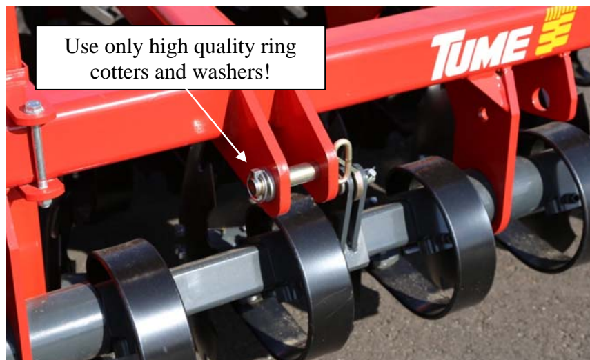
Figure 1. A washer must be installed under the ring cotter due to the oval shape of the tow lug holes
