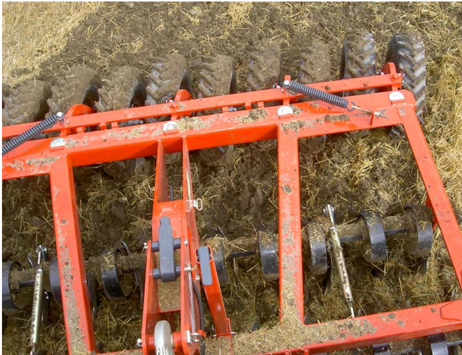
Figure 11. Hinged support wheels allow end turns without raising the cultivator
