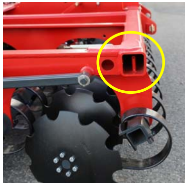
Figure 5. Additional weights can be inserted in the front beam of the cultivator
