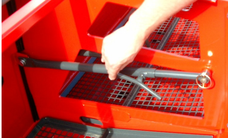
Picture 8. The adjusting rod of the hopper's dividing wall
